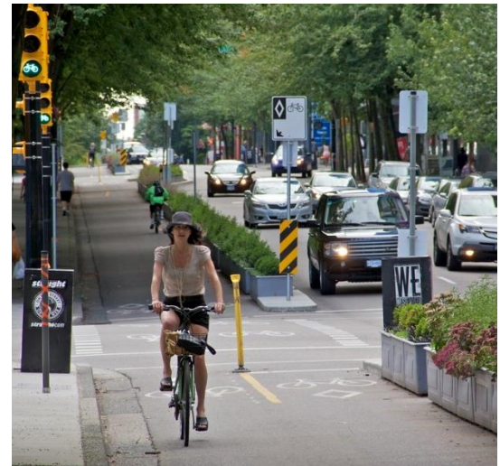
Hornby Street in Vancouver, BC, is an example of utilizing planters to create a separated bicycle route.
